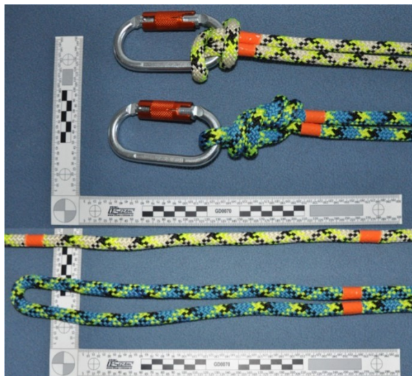
Figure 7: Comparison of figure eight loop and Polish knot rope consumption
