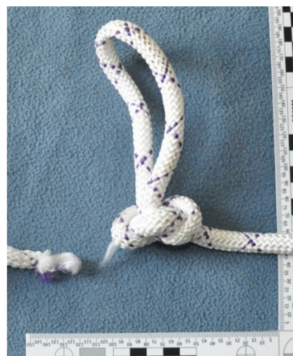
Figure 4: The undamaged loop after Test 0-a [2, p. 6]
