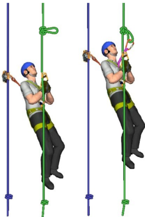
Figure 1: Clipping to the loop when passing the knot [2, p. 1]
