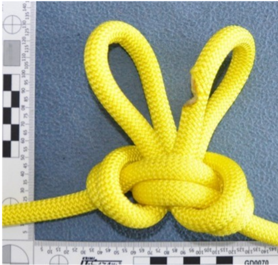
Figure 16: The double alpine butterfly is safe enough clipping cowstail even if one of the loops is damaged [2, p. 17]
